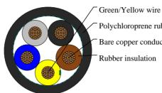
Polychloroprene rubber outer jacket Bare copper conductor
